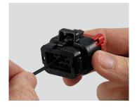
Step 3: Insert the contact into the connector cavity until there is an audible and tactile click. A slight tug will verify the contact is locked in place.
