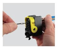
**Step 3:** Pull contact wire assembly out of connector.
