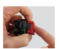
**Step 4:**After all the contacts have been inserted, close the wedgelock by simultaneously squeezing locking latches inward and pushing the wedgelock into the housing.
