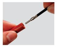
**Step 2:** Hold Jiffy Splice between thumb and forefinger approximately one half inch behind cavity.
