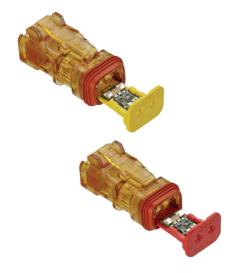
The Detector connector has an integrated LED used for diagnostics. The transparent housing features reduced diameter seals and may be ordered with or without an end cap. Color coded wedgelocks for operating voltages, 12VDC and 24VDC are available.
