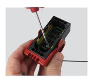
**Step 4:** Unlock the contacts and pull on the wire.
