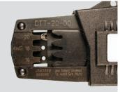
Step 1: Cycle the hand tool to the open position. Place the contact into the correct die nest.
