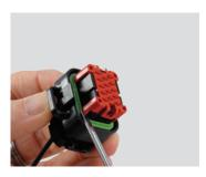
Step 1: Insert the tip of a screw-driver (2-5mm wide blade) between the edge of the plug assembly housing and one corner of the wedgelock.
