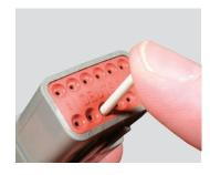
**Step 2:** With perpendicular motion, apply downward pressure to the small diameter end of the sealing plug.
