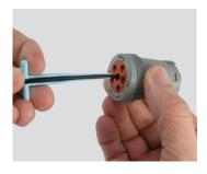
Step 1: With rear insert toward you, snap appropriate size removal tool over the wire of contact to be removed.
