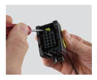
**Step 1:**Using a DT-RT1 or a screwdriver, unlock the integrated secondary lock.
