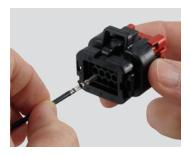
**Step 2:** Check that the wedgelock of the plug assembly is in open position. Align the contact with the applicable cavity.
