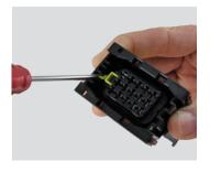
**Step 3:**Push the integrated secondary lock into the locked position with a DT-RT1 or a screwdriver.
