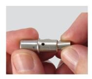
**Step 1:** Place crimp sleeve reducer into contact barrel.
