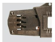
**Step 2:**Partially close the tool until the contact is held in place.
