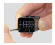
Step 2: Insert the tool into the contact cavity and deflect the contact retention finger.
