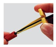
**Step 1:**Snap appropriate size removal tool over the wire.
