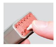
Step 2: With perpendicular motion, apply downward pressure to the large diameter end of the sealing plug.
