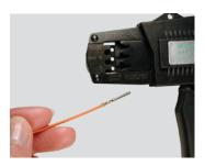
**Step 4:**Close the tool until the ratchet releases. The ratchet is released when a loud click is heard and crimp is complete.
