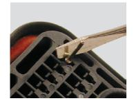
**Step 2:**To remove contacts, gently pull wire backwards, while at the same time releasing the locking finger by moving it away from the contact with a screwdriver.
