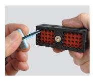
**Step 2:**Slide tool along the wire into the insert cavity until it engages contact and resistance is felt.
