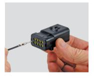
**Step 3:** Align the contact with the desired circuit cavity at the rear of the housing assembly.
