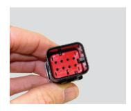
**Step 2:** Verify the PLR is in the pre-staged position, unlocked.
