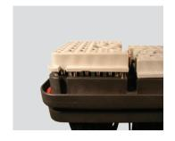
**Step 2:** If the wedgelock will not go all the way in, check to make sure all of the contacts are properly seated.
