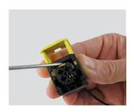
**Step 4:**Push the integrated secondary lock into the locked position with a DT-RT1 or a screwdriver.
