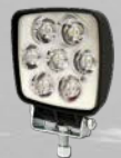
EW2112-DEU SEVEN 1-WATT LEDs 12-80V | Flood | 1,000 Lumens Deutsch connector CE, R10, UL, IP67, RoHS
